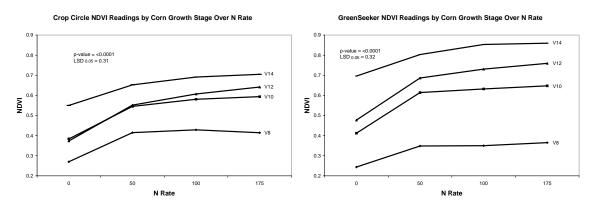
Figure 1. Crop Circle<sup>™</sup> and GreenSeeker<sup>™</sup> NDVI readings at corn growth stages V8, V10, V12, and V14 as affected by N rate.
